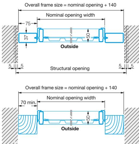
Fitting in the opening requires that the given dimensions be adhered to with greater accuracy.
