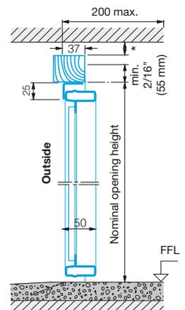
\* 40 mm headroom required for electric operator
