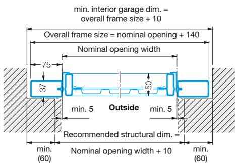
Behind opening installation with the Hörmann steel frame allows for a wider range of structural openings to be spanned, this can be particularly helpful with non-standard openings which would normally require special sized doors. The diagrams show the minimum tolerances that should be adhered to. PLEASE NOTE: the overall frame sizes are shown as additions to the nominal opening sizes.
