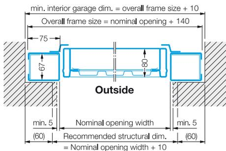
The recommended structural dimensions are recommended planning dimensions. Minimum sideroom, headroom and opening sizes are all based on these dimensions.
