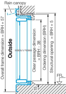
Single leaf door (supplied with bottom threshold as standard, will be removed on site)
