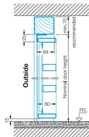
Fitting in the opening requires that the given dimensions be adhered to with greater accuracy.
